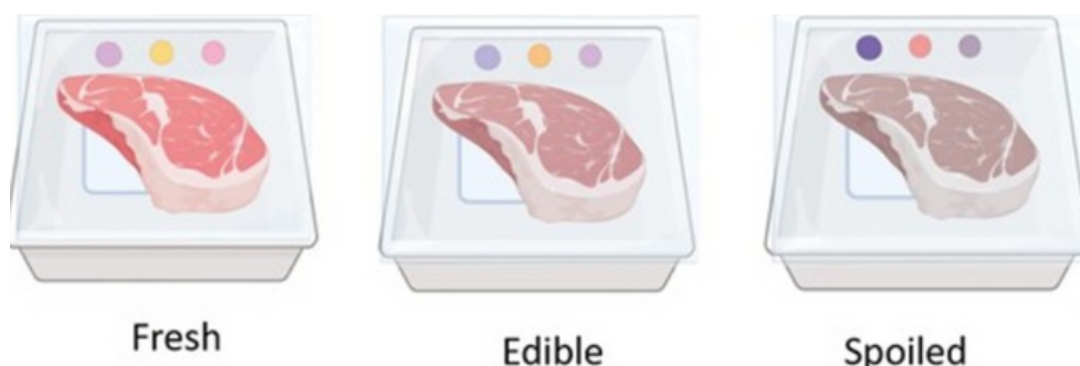
Fig. 2.c. An example of a label whose color changes as meat quality degrades.
